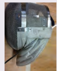
An example of a near miss incident- blade penetrated protective clothing, luckily no injury occurred to fencer.
